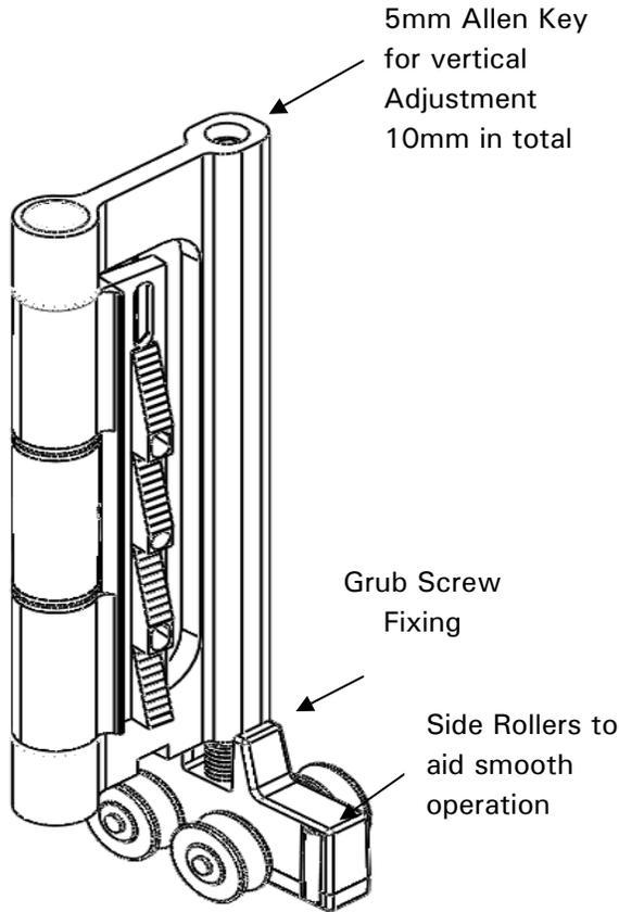
The double leaf roller incorporates a hinge which fixes the roller to the door sashes (top & bottom rollers) the rollers themselves have 10mm of adjustment (+ &- 5mm).
