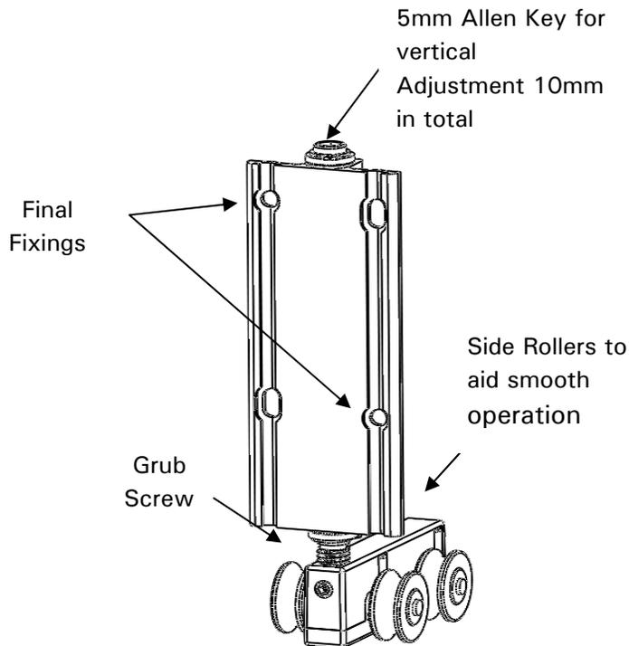
The single leaf roller is screwed directly in to the door sash euro-groove (top & bottom rollers) the rollers themselves have 10mm of adjustment (+ &- 5mm).
