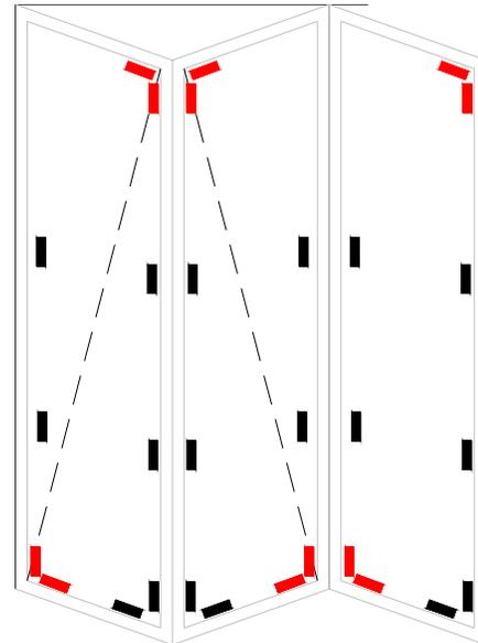
**█** PACKING TO PREVENT GLASS SLIPPAGE AND PROVIDE STIFFNESS TO THE DOOR.
