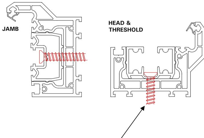
If this fixing is over tightened, it will distort the aluminium roller case and prevent the door from operating as it should.
